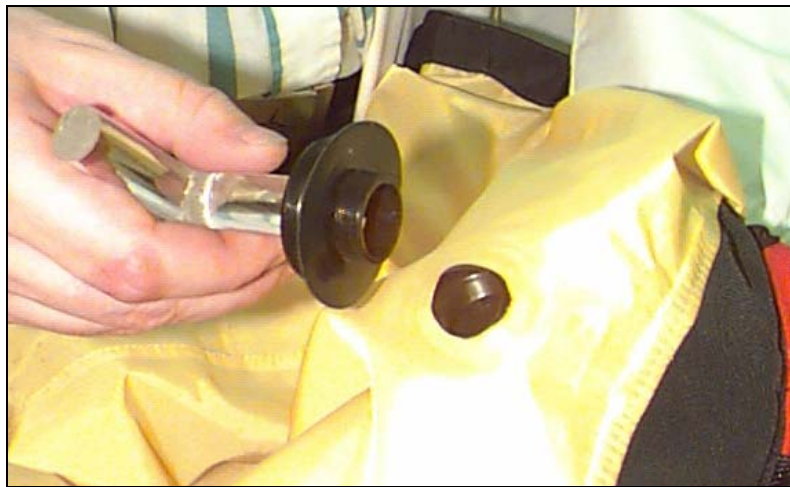
Figure 25. Step c. Exhaust Valve Replacement
