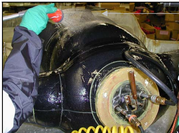
Figure 25. Step g. (Suit Leakage Test)
