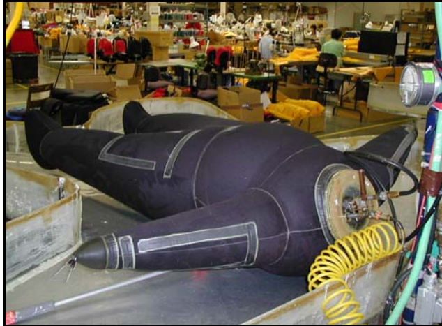
Figure 24. Step f. (Suit Leakage Test)
