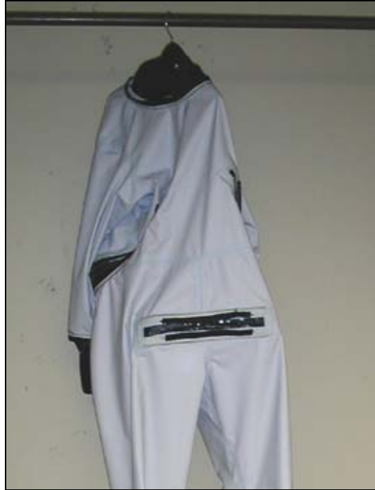
Figure 28. Step j. Suit Leakage Test
