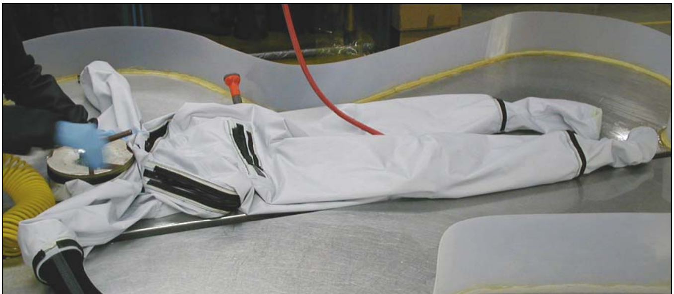
Figure 20. Step a. Suit Leakage Test
