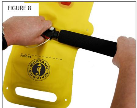
Step 2 - Remove the handle, containing the discharged CO<sub>2</sub> cylinder, by firmly rotating counter-clockwise (Fig. 8). To ensure that you do not re-install a used cylinder, discard immediately. If cylinder is discharged, replace with new handle. Ensure the cylinder has not been pierced. See RE-ARMING.
