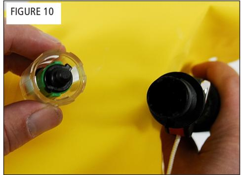
Step 4 - Remove the bobbin from the cap. Discard the bobbin. Check the housing to be sure it is clear of debris, clean and dry (Fig. 10).
