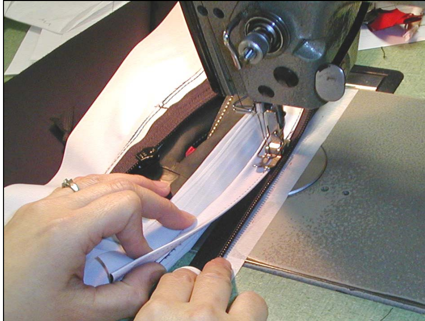
Figure 50. Step d. Interconnection Zipper Replacement
