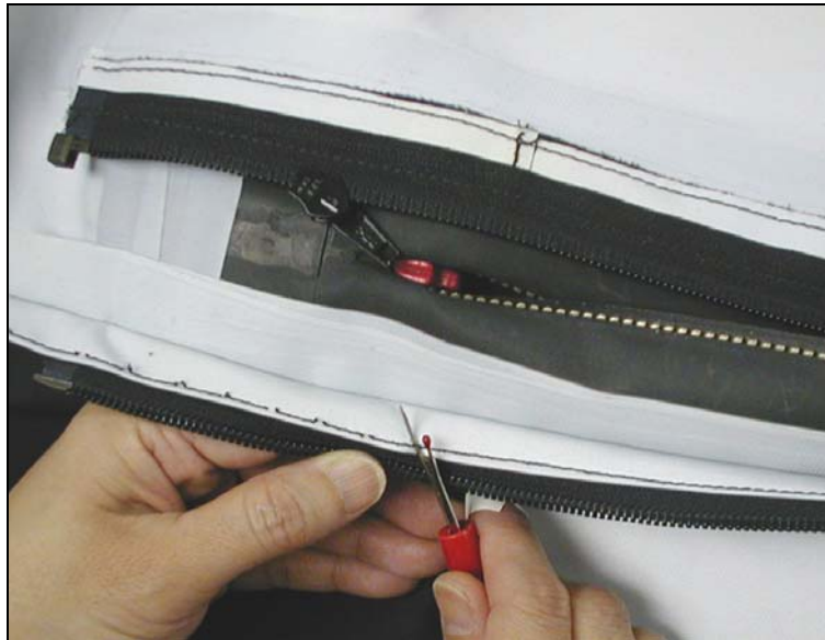
Figure 48. Step b. Interconnection Zipper Replacement
