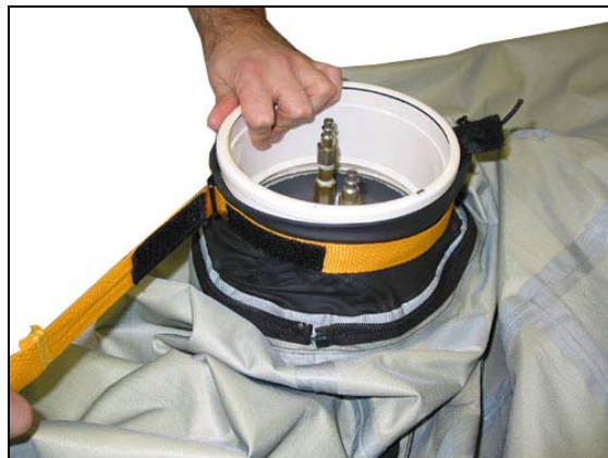
Figure 34. Step f. Suit Leakage Test
