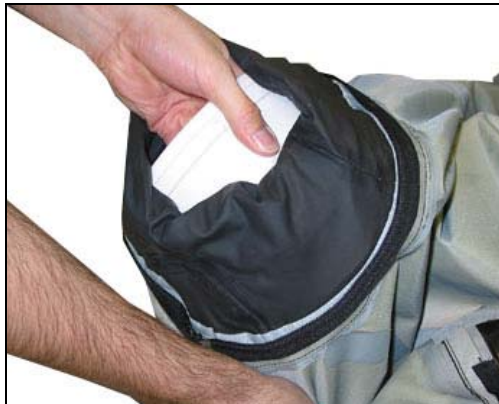
Figure 31. Step c. Suit Leakage Test
