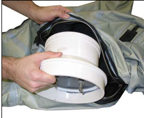
Figure 30. Step b. Suit Leakage Test
