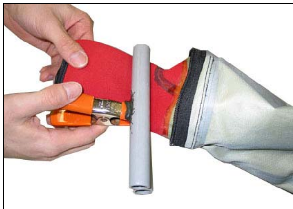
Figure 35. Step g. Suit Leakage Test
