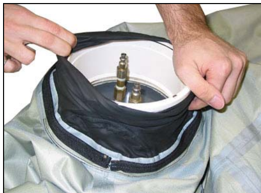
Figure 30. Step d. Suit Leakage Test
