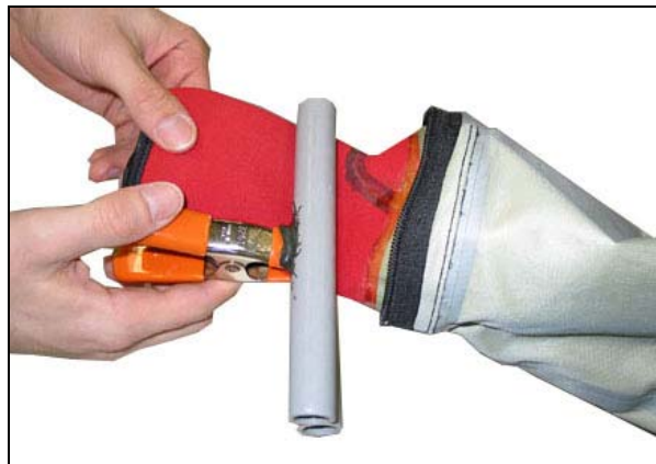
Figure 33. Step g. Suit Leakage Test
