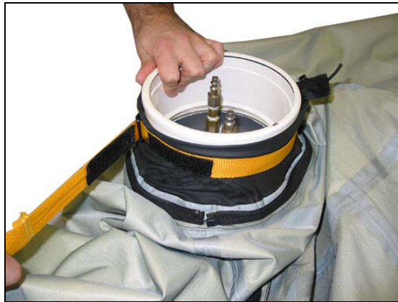
Figure 32. Step f. Suit Leakage Test
